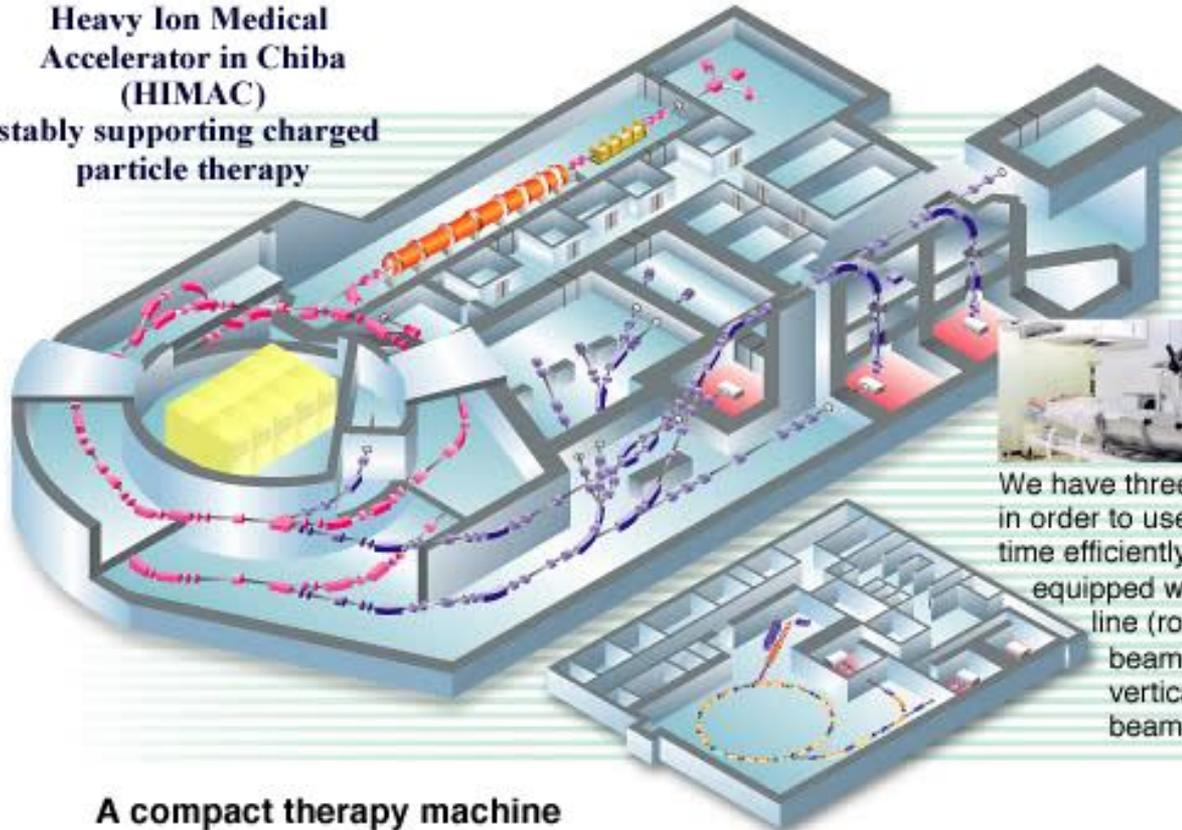
We have three treatment rooms in order to use the HIMAC beam time efficiently. These rooms are equipped with a vertical beam line (room A), a horizontal beam line (room C) and vertical and horizontal beam lines (room B).
