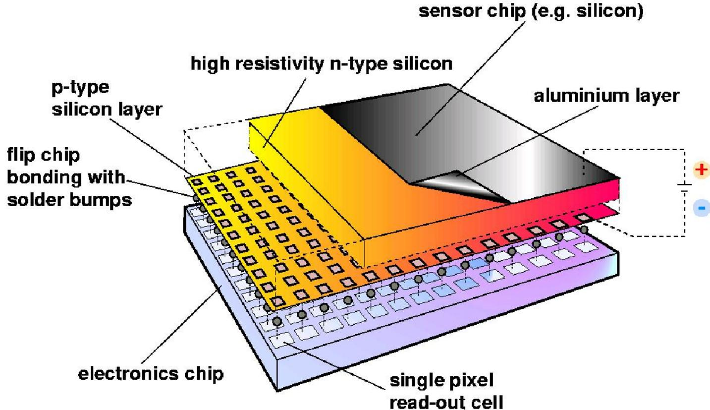
**Detector and electronics readout are optimized separately**
