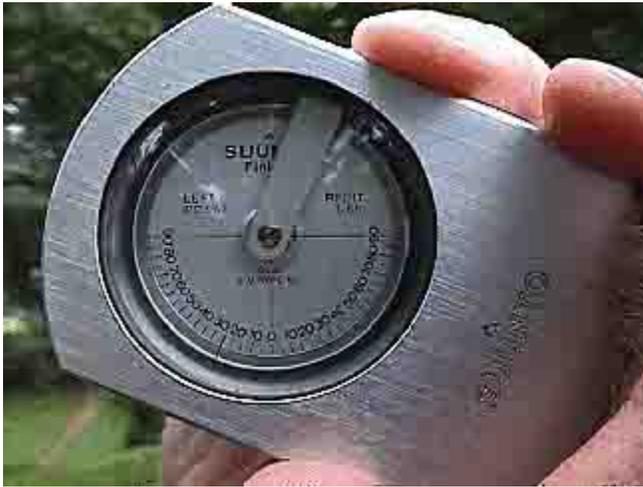
A clinometer is used by foresters to measure the height of a standing tree. It works using principles of angles and geometry.
