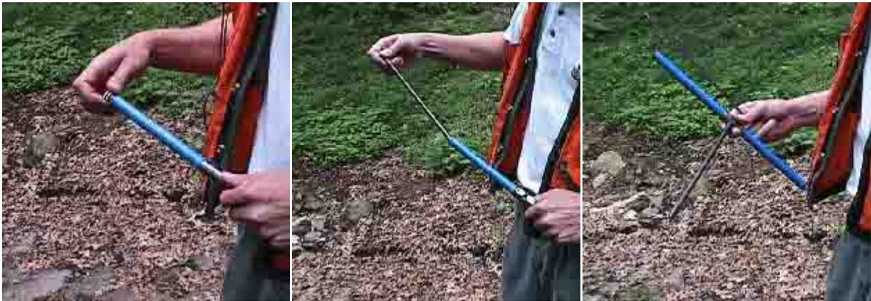
An increment borer is used to determine the age of a tree. The borer is compact so it can fit into a pocket of the vest and is easily assembled.
