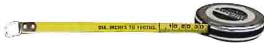
A diameter tape (D-tape) is used by foresters to measure the diameter of a tree. Since trees are swelled at the base, measurements are made 4.5 feet above the ground in order to give an average diameter estimate. The D-tape is wrapped around a tree and is specially designed to convert the tree circumference to tree diameter.
