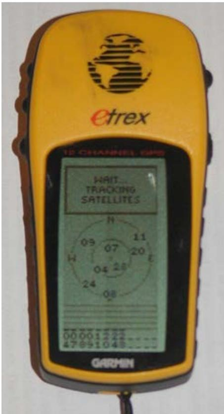
The GPS unit above is a Garmin etrex that provides the user with the necessary tools to obtain latitude, longitude, elevation, and the ability to mark and save routes. GPS is used for a variety of purposes. Its uses are found everywhere from the military to inside peoples' cars as a navigation system.
