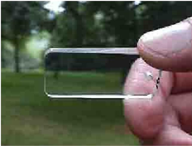
A prism is used to help determine whether or not an area has too many or too few trees. Using geometry, the number of trees and the size of the trees, this instrument estimates the density of trees in square feet per acre. This information can be used to determine tree volume and proper management strategies.
