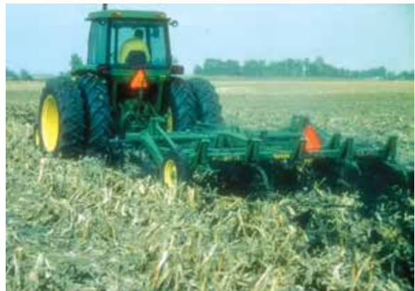
Figure 16.3. Left: Moldboard plowing inverts a sod and leaves no surface protection. Right: Chisel plow shanks till soil and leave some residue cover.
