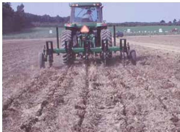
Figure 15.5. Left: Subsoiler shank provides deep compaction relief (wings at the tip provide lateral shattering). Right: Zone building provides compaction relief and better rooting with minimal surface disturbance. Right photo by George Abawi.
