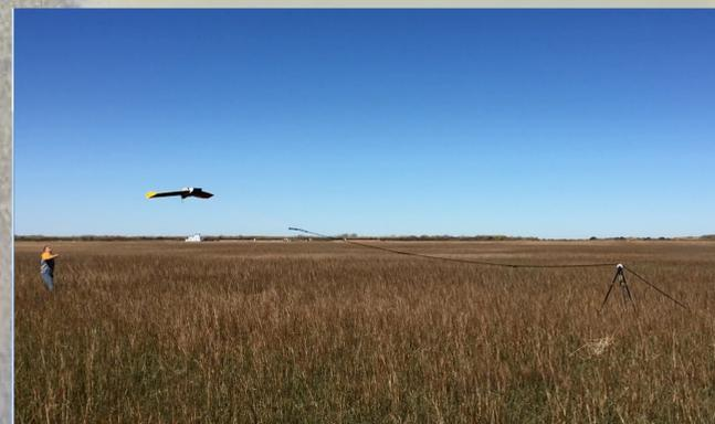
Figure 6. The QUESTUAV Aqua Drone being launched in Bastrop Bay using the pulley and bungee cord launching system.
