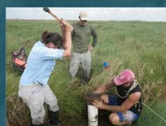
Figure 6. Team using a king sampler to get sediment core, (also important team trust building exercise)
