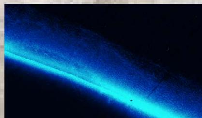
Fig 4. Mosaic of the sonar images collected using the side-scanning sonar system. The processing is conducted using SonarTRX software.
