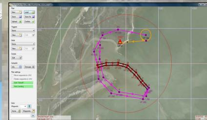
Fig 6. A flying acquisition plan in the Bastrop Bay shows the flying path that includes the launching and navigation part, surveying path along the reef and the navigation part to landing.
