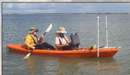
Fig 3. Operating the side-scanning sonar system in shallow water from a kayak.
