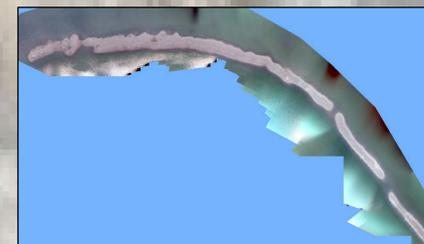
Fig 8. 2D orthoimage of the data acquired using UAV at 200ft altitude; the spatial resolution is 2.2.
