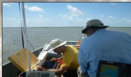
Fig 2. Operating the side-scanning sonar system with a transducer installed in the front of a small vessel.
