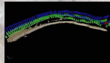
Fig 7. Densified point cloud: green dots indicate where the UAV is, blue dots where the UAV should be at the time of the image capture, and red dots indicate discarded data.
