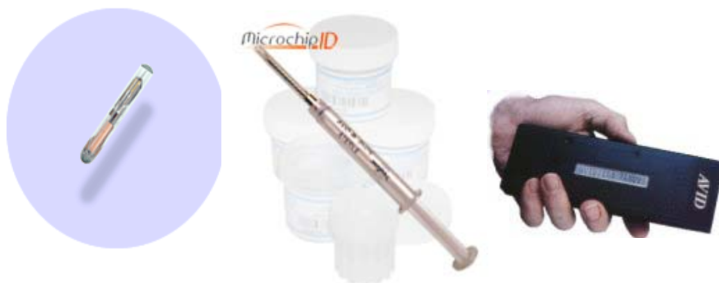
Figure 6. Avid PIT tag, injector, and reader used to identify terrapins.
