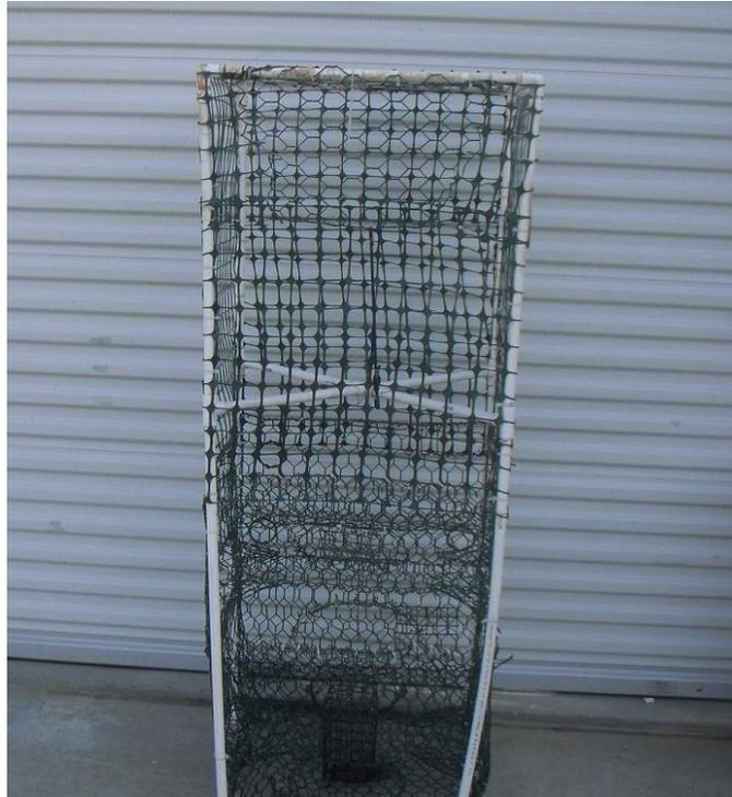
**Figure 8. Modified crab traps, designed by Emma Clarkson. The base of the modified trap is made from two crab traps on top of each other. The top was removed from the bottom trap and the bottom and top were removed from the top trap to create one large open space with 8 points of entry.**
