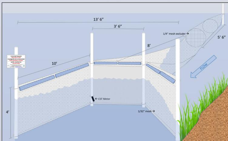
Figure 3. Fyke net design and specifications used to sample for glass and elver American Eel.
