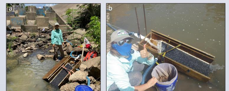
Figure 6. a: Gravity-fed eel ramp deployed at a tributary to Greens Bayou in Houston. b: ramp deployed at steep bank creek, a tributary to the Brazos River in Fort Bend, County.
