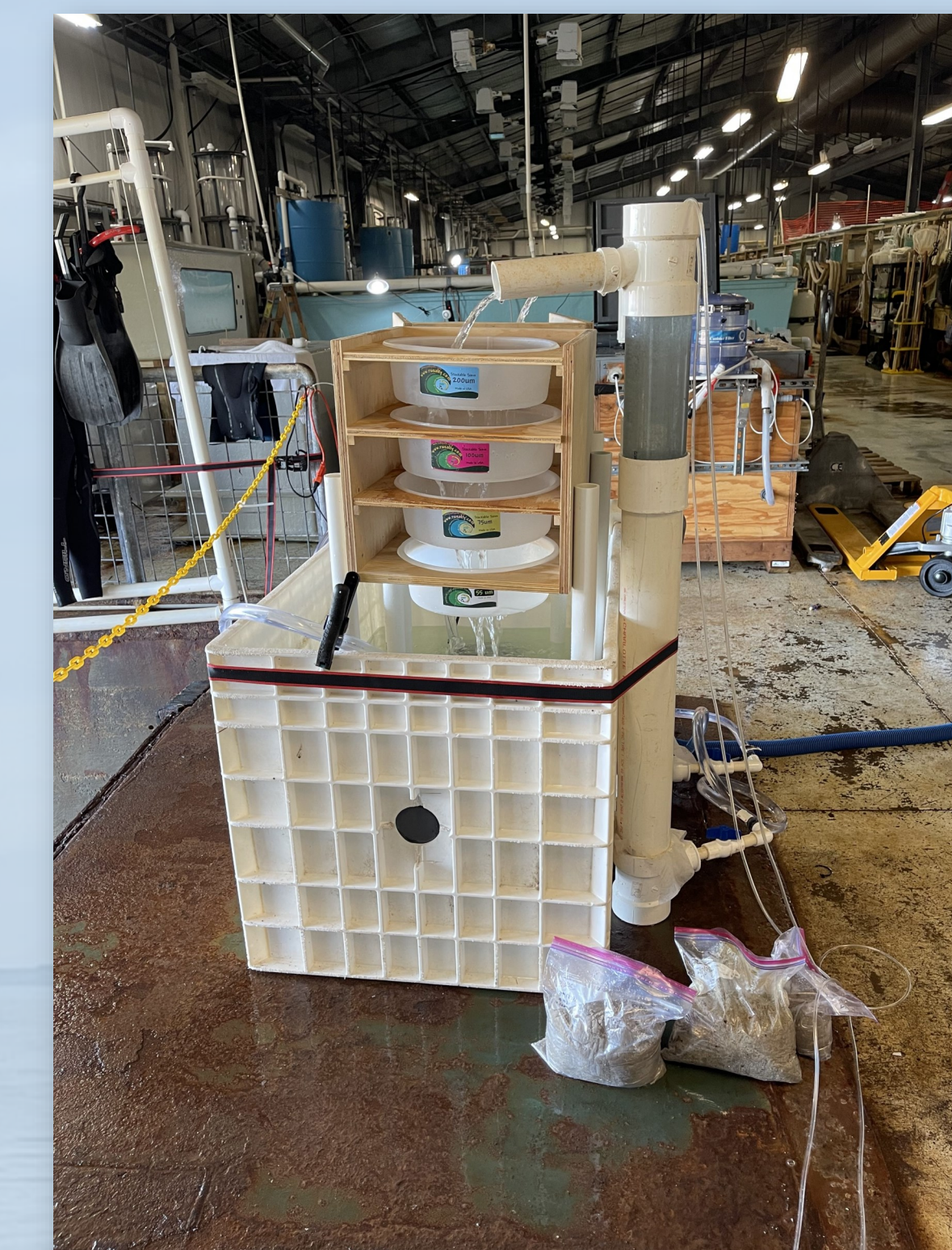
Figure 4. Density separator apparatus as described in Sartain et al. (2018), shown here assembled for a TIRN outreach event. Sieves are stacked in descending mesh size (200 > 100 > 75 > 55 µm) to prevent clogging of mesh, and all material is collected for microscopic analysis.
