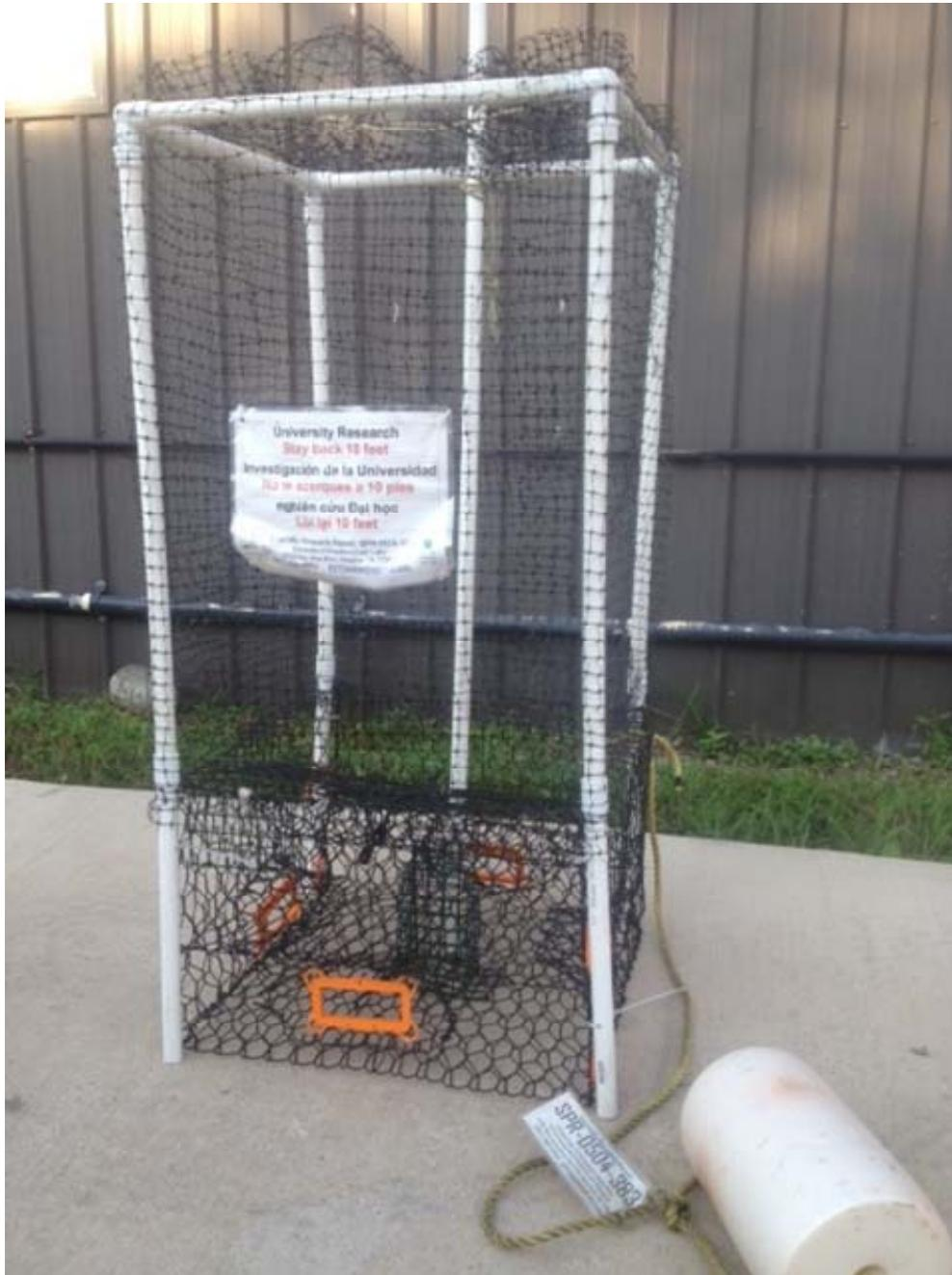
**Figure 18. Experimental crab pot with escape chimney used to test various BRD devices at all sites except the Trinity site. Note orange BRD devices installed on this trap.**
