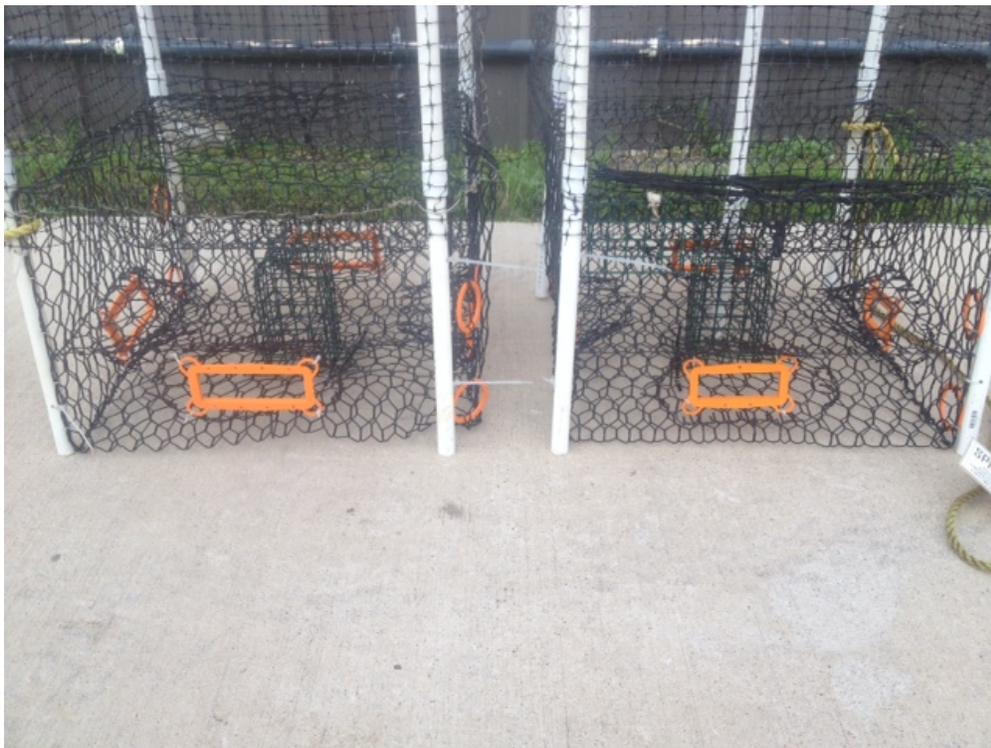
**Figure 20. Comparison of large (left) and small (right) BRDs evaluated during the study.**
