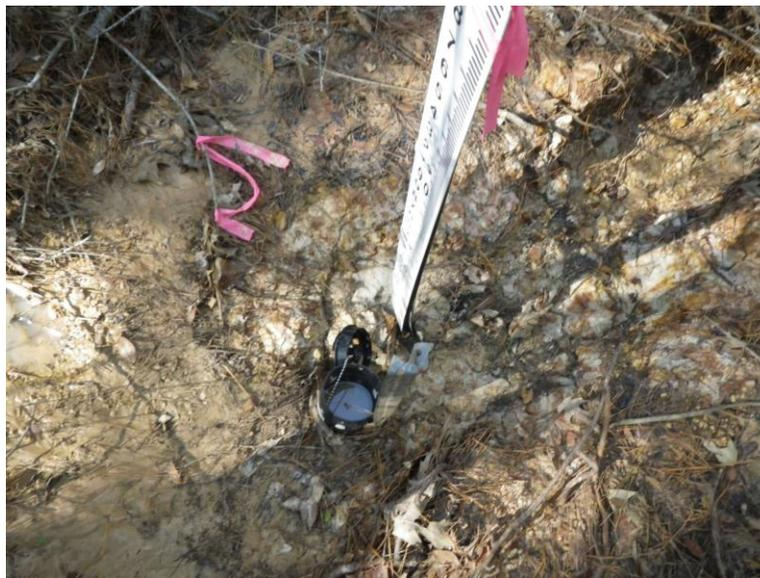
**Figure 82. Photograph of stormwater sampler at site 2 on November 29, 2011 prior to stormwater sampler removal on last day of study. (Source: hand held camera). No stormwater sample bottle had been deployed prior to this event.**
