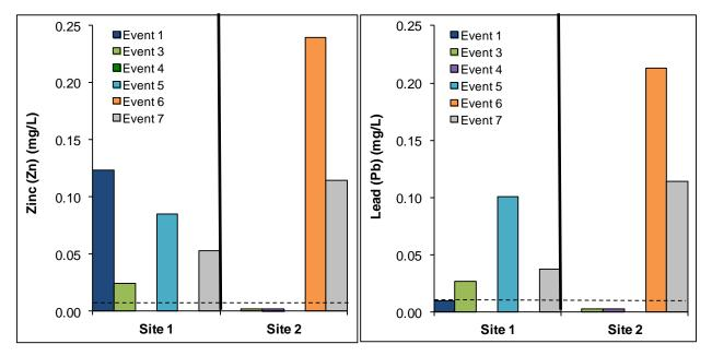
Figure 33. Zinc and lead levels for rainfall events. Dashed line represents detection limit for this test (< 0.01 mg/L); values below this line indicate presence at levels below the detection limit. Grab samples only.
