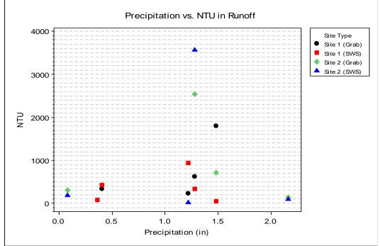
Figure 27. Relationship between precipitation and turbidity (NTU) levels in runoff at each site by collection method. There was no significant (p <0.01) linear relationship between variables.
