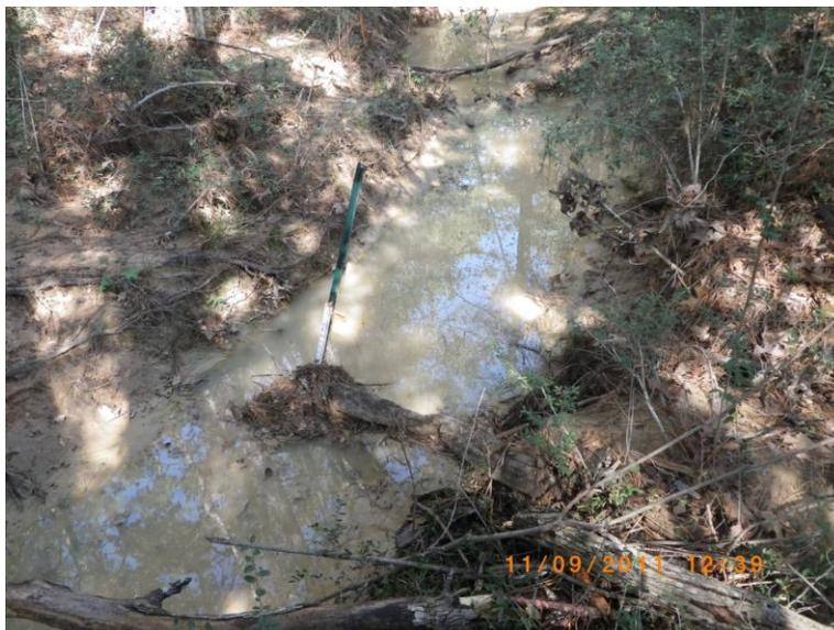
**Figure 58. Photograph of site 1 taken on November 9, 2011 showing stormwater sampler and staff gage with accumulated debris (Source: hand held camera). No sample bottles deployed prior to this rain event.**
