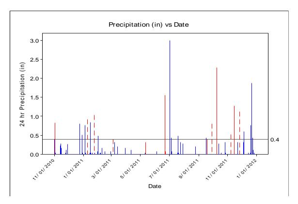
Figure 12. Recorded 24 hour precipitation at the HCFCD 1050 rain gage co-located at the USGS 08068500 site on Spring Creek and I-45. Red lines denote dates when sampling was conducted at the site. Dashed red lines denotes dates when unsuccessful sampling attempts were made on that date or afterwards. The horizontal reference line is the 0.4 inch decision level for sampling when combined with 72 previous hours of dry weather.
