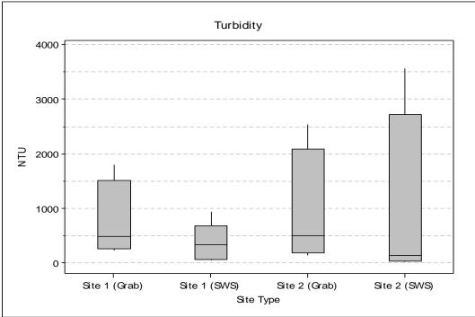
Figure 25. Boxplot of turbidity (NTU) levels measured at each site and type of sample over all sampling periods of the study
