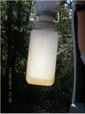
Figure 72. Photograph of collection bottle from stormwater sampler bottle at site 2 on November 9, 2011, a day after rainfall. (Source: hand held camera). Note minimal sample volume collected which was not used for analyses.
