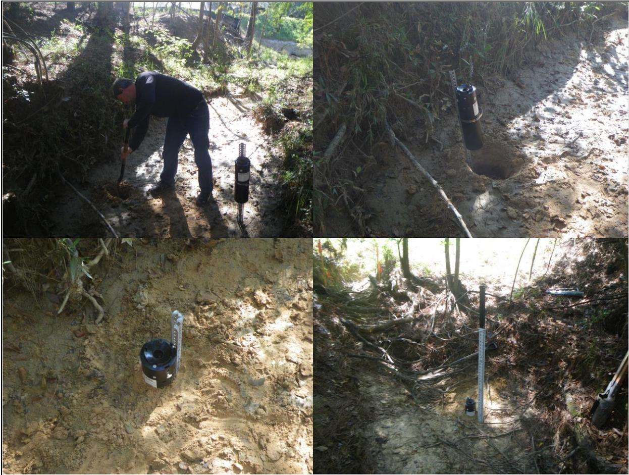
Figure 9. Deployment of the stormwater sampler used during this study.
