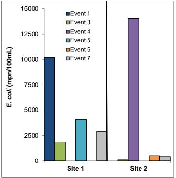
Figure 28. *E. coli* levels in runoff during rainfall events. Data based on grab samples only.
