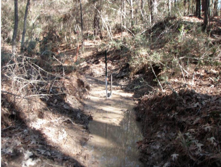
**Figure 36. Photograph of site 1, taken during wet weather event 1 on 11/2/10, looking downstream at stormwater sampler and gage. (Source: automated game camera).**
