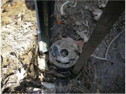
Figure 44. Photograph of site 1, taken on 2/8/11, depicting stormwater sampler with sediment caked on sampler tube top (Source: hand held camera). Sampler checked after non-qualifying rain event.
