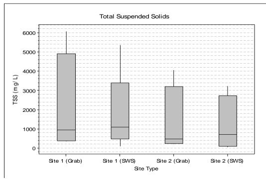
Figure 24. Boxplot of total suspended solids (TSS) levels measured at each site and type of sample over all sampling periods of the study.
