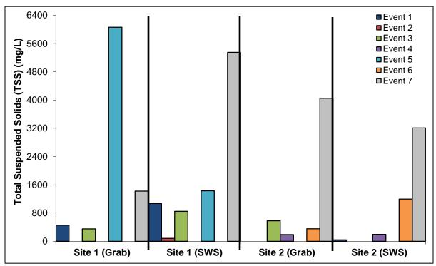
Figure 22. Total suspended solid levels in runoff during rainfall events. Grab = grab samples; SWS = stormwater sampler.
