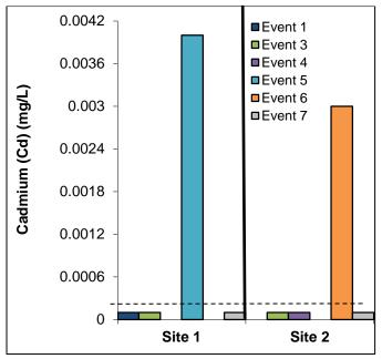
Figure 32. Cadmium levels for rainfall events. Dashed line represents detection limit for this test <0.0001 mg/L); values below this line indicate presence at levels below the detection limit. Grab samples only.
