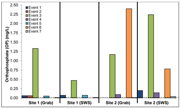
Figure 19. Orthophosphate levels in runoff during rainfall events. Dashed line represents detection limit for this test (<0.02 mg/L); values below this line indicate presence at levels below the detection limit. Grab = grab samples; SWS = stormwater sampler.
