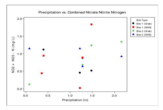
Figure 18. Relationship between precipitation and combined nitrate nitrite nitrogen runoff levels at each site by collection method.
