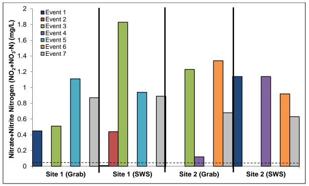
Figure 14. Nitrate and nitrite nitrogen levels in runoff during rainfall events. Dashed line represents detection limit for this test (<0.04 mg/L); values below this line indicate presence at levels below the detection limit. Grab = grab samples; SWS = stormwater sampler.
