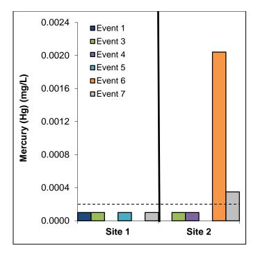
Figure 31. Mercury levels for rainfall events. Dashed line represents detection limit for this test (<0.0002 mg/L); values below this line indicate presence at levels below the detection limit. Grab samples only.
