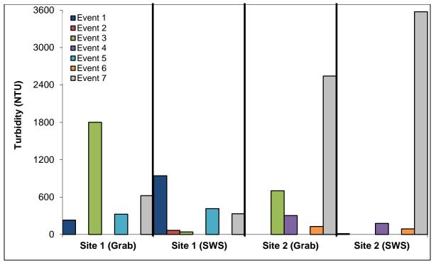
Figure 23. Turbidity levels in runoff during rainfall events. Grab = grab samples; SWS = stormwater sampler.
