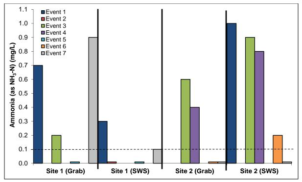
Figure 13. Ammonia nitrogen levels in runoff during rainfall events. Dashed line represents detection limit for this test (<0.01 mg/L); values below this line indicate presence at levels below the detection limit. Grab = grab samples; SWS = stormwater sampler.
