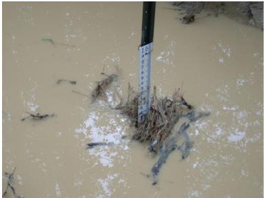
Figure 61. Photograph of site 1 taken during stormwater sampling event 5 on September 19, 2011 showing stormwater sampler obstructed with debris (Source: hand held camera).
