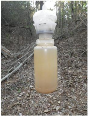
Figure 56. Photograph of site 2 taken on August 18, 2011 showing stormwater sampler bottle completely full from non-qualifying wet weather event (Source: hand held camera).
