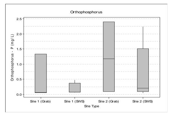
Figure 20. Boxplot of orthophosphorus levels measured at each site and type of sample over all sampling periods of the study.
