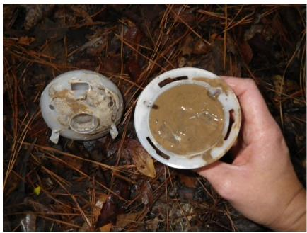
Figure 78. Photograph of sediment deposited on the stormwater sampler collector at site 2 during event 7 on November 15, 2012. Note cap lying on the ground had a frothy film on it. (Source: hand held camera).
