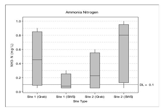
Figure 15. Boxplot of ammonia nitrogen levels measured at each site and type of sample over all sampling periods of the study.
