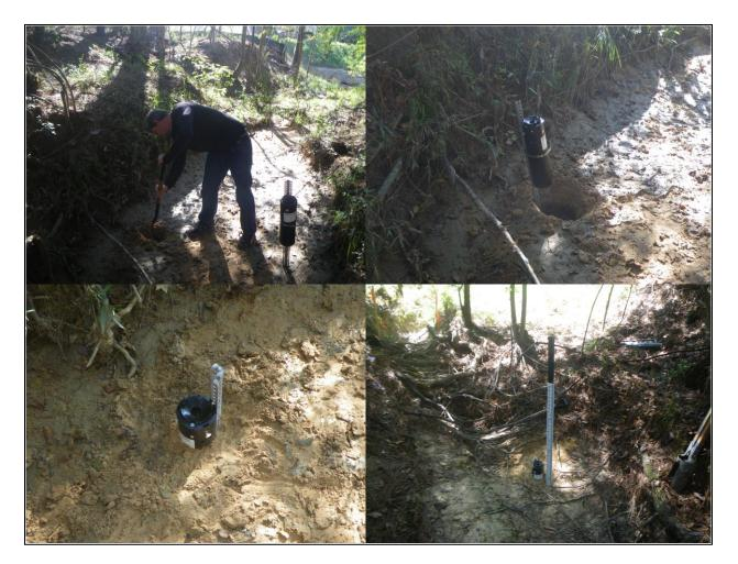
Figure 9. Deployment of the stormwater sampler used during this study.
