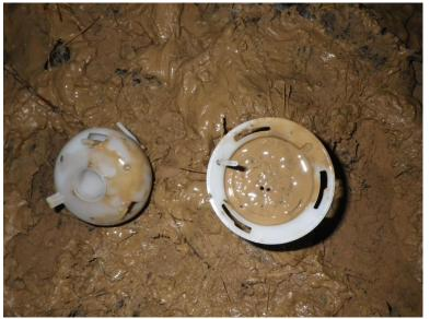
Figure 74. Photograph of stormwater sampler at site 1 during sampling event 7 on November 15, 2011. (Source hand held camera). Note sampler cap is full of mud.
