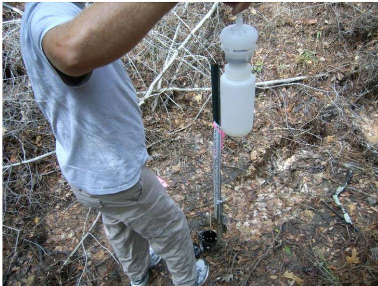
**Figure 64. Photograph of site 2 taken on stormwater sampling event 5, September 19, 2011 showing minimal water in ditch and minimal amount of water in sampler (Source: hand held camera). Insufficient water collected for most analyses.**
