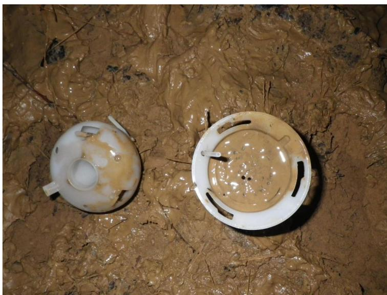
**Figure 74. Photograph of stormwater sampler at site 1 during sampling event 7 on November 15, 2011. (Source hand held camera). Note sampler cap is full of mud.**
