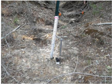
Figure 55. Photograph of site 2 taken on August 18, 2011 showing stormwater sampler and gage in dry creek (Source: hand held camera).
