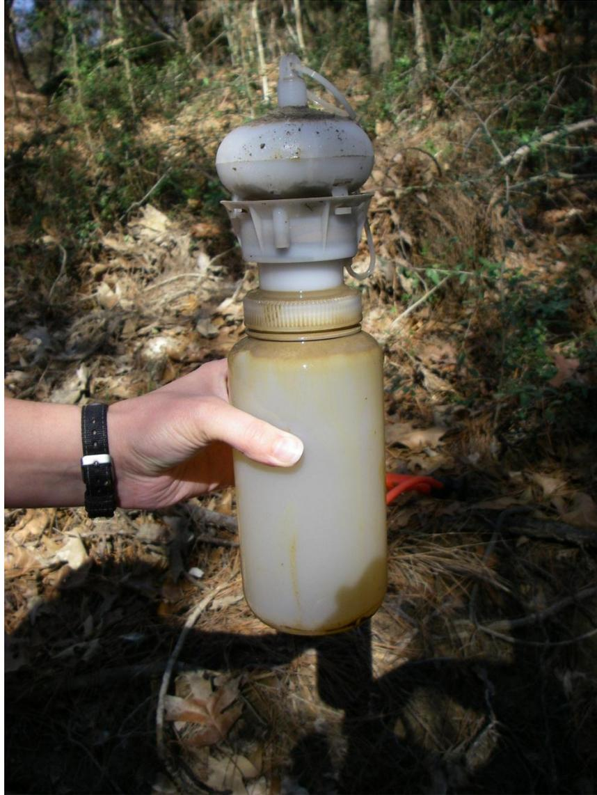
**Figure 45. Photograph of site 1, taken on 2/8/11, depicting stormwater sampler bottle completely filled after a non-qualifying rain event (Source: hand held camera).**
