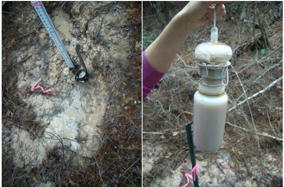
Figure 77. Photograph of the staff gage and sampler at site 2 on November 15, 2012, with sampler cap removed; more sediment deposited in the creek from the construction. Note rain water filled the sampler (Source: hand held camera).
