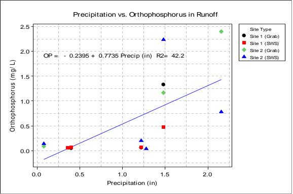
Figure 21. Relationship between precipitation and orthophosphorus levels in runoff at each site by collection method. Slope of regression line was significant at p = 0.009.
