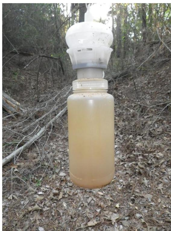
**Figure 56. Photograph of site 2 taken on August 18, 2011 showing stormwater sampler bottle completely full from non-qualifying wet weather event (Source: hand held camera).**
