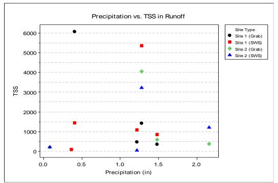
Figure 26. Relationship between precipitation and total suspended solids (TSS) levels in runoff at each site by collection method. There was no significant (p <0.01) linear relationship between variables.
