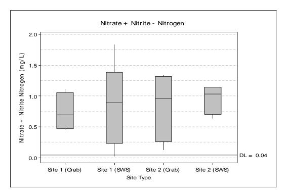
Figure 16. Boxplot of nitrate + nitrite nitrogen levels measured at each site and type of sample over all sampling periods of the study.
