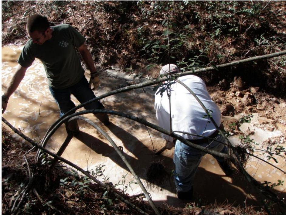
**Figure 41. Photograph of site 1, taken on 1/28/11, depicting HCFCD personnel digging up stormwater sampler to move it downstream (Source: hand held camera). Sampler was buried in mud.**
