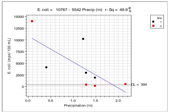
Figure 29. Relationship between precipitation and *E. coli* (mpn/100 mL) levels in runoff at each site. Significant at (p = 0.05) linear relationship between variables. CL = TCEQ criteria level.
