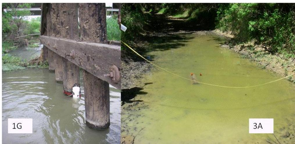
**Figure 24. PVC and lock box data sonde deployment methods, sites 1G (left) and 3A (right).**
