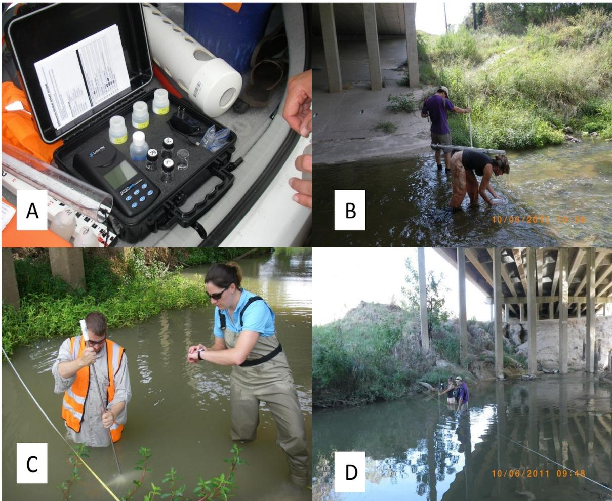
**Figure 25. (a) Portable turbidity meter for field NTU readings; (b) field personnel taking depth and grab samples; (c) field personnel taking SSC samples; (d) field personnel taking flow measurements and sonde readings**
