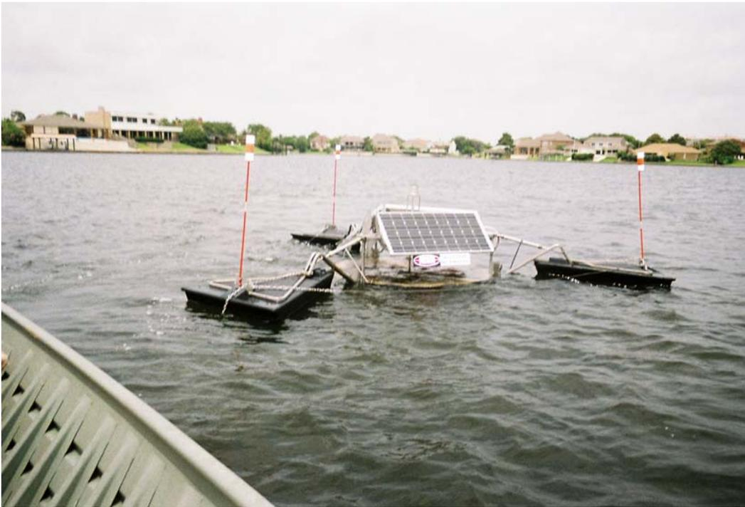
Figure 4. Solar powered aerator assembly floating in middle of Lake Madeline.
