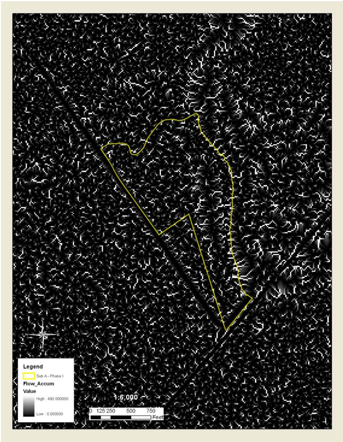
Figure 4. Estimated flow accumulation using the ArcGIS™ extension Arc Hydro™ and the TSARP DEM. Areas in white represent the areas most likely to accumulate surface water.
