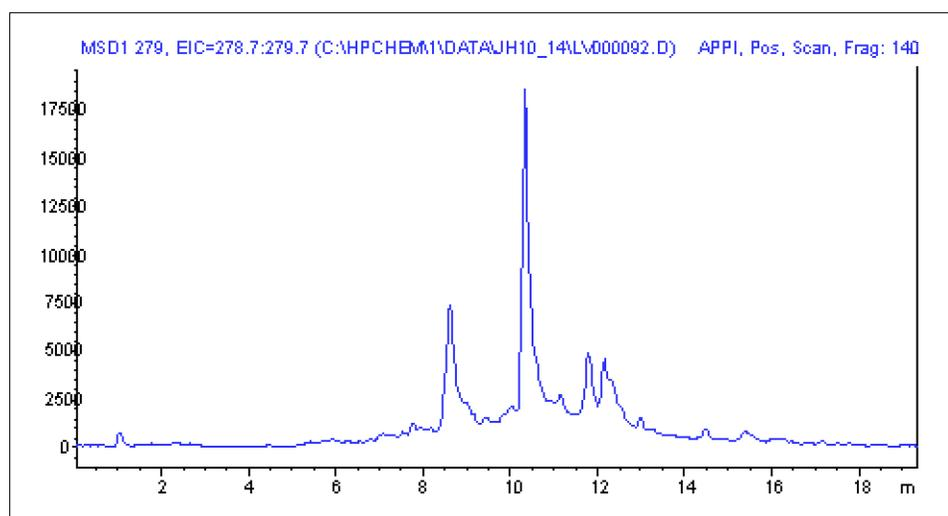
**Figure 1. Extraction of m/z 279 Ion in the Effluent of a Simulated Bioprocess Water Recovery System**
