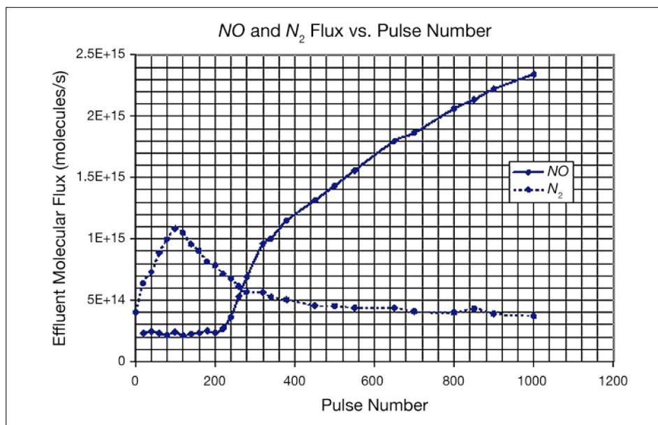
Figure 2. Dependence of Effluent Flux of  $\text{N}_2$  and  $\text{NO}$  During the Sequential Pulsing of  $\text{NO}$  Over an Initially Oxidized  $\text{Pt}/\text{BaO}/\text{Alumina}$  Catalyst
