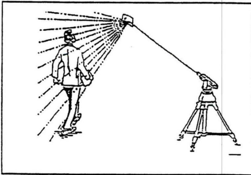
Diffuse reflection is less hazardous than specular.
