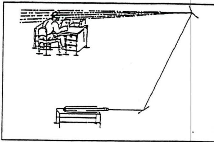
Curve-surface specular reflections are less hazardous than flat surface specular reflections.
