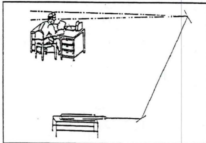
Specular reflections are most hazardous when the reflecting surface is flat or concaved.
