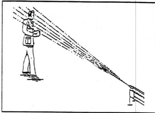
A direct interbeam viewing is most hazardous.
