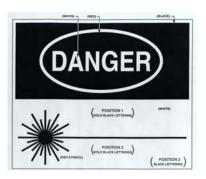
Sample Warning Sign for Class IIIb and Class IV Lasers
